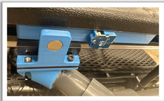
Figure 4: The hall effect sensor mounted in the custom 3-D printed bracket. The magnet that is used to activate the sensor and send signals to the motor is shown on the left, mounted on the moving slider.
