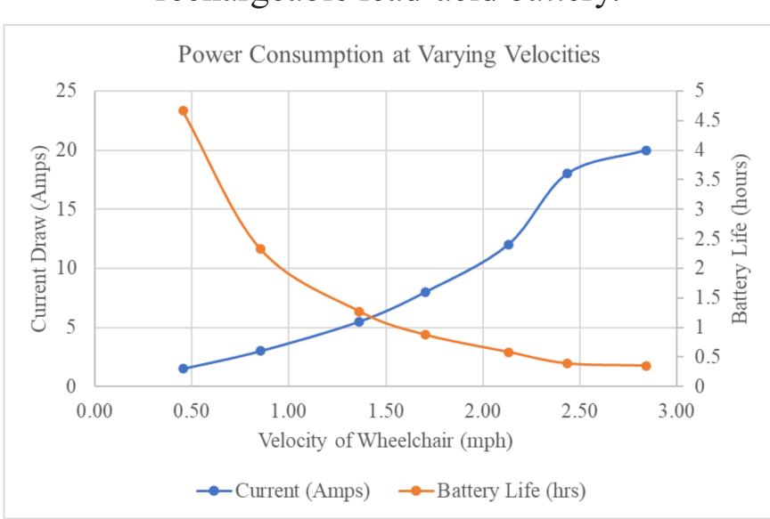
Fully Electric State → Operates at 1 mph for ~2 hours Manual Input → Max Speed at 3 mph for ~20 minutes
